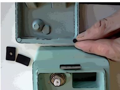
Remove the small circular sections from the center of the rectangular adhesive neoprene pads.
