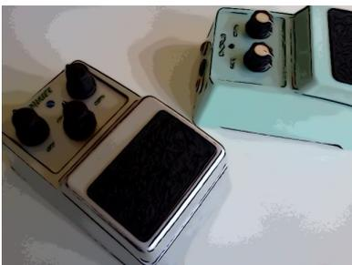
Test that the switch clicks just before the pedal closes. If it clicks with more than 2mm of travel left, adjust the switch to a lower position.
